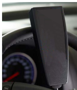
Wireless transmission EOBD scan tool.
